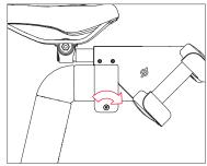
▲ WARNING: Do not over-tighten the seat slider adjustment knob. Over-tightening could result in malfunction or breakage.
