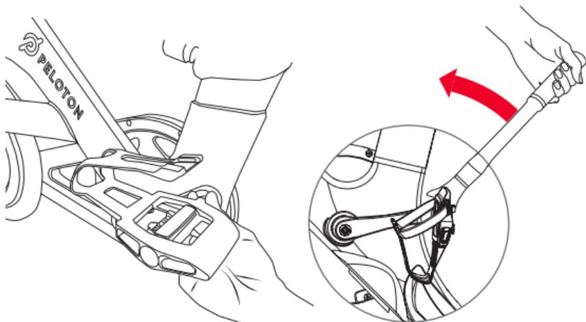
Tighten pedals regularly. Remember to turn the wrench toward the front of the bike to tighten on both sides.
